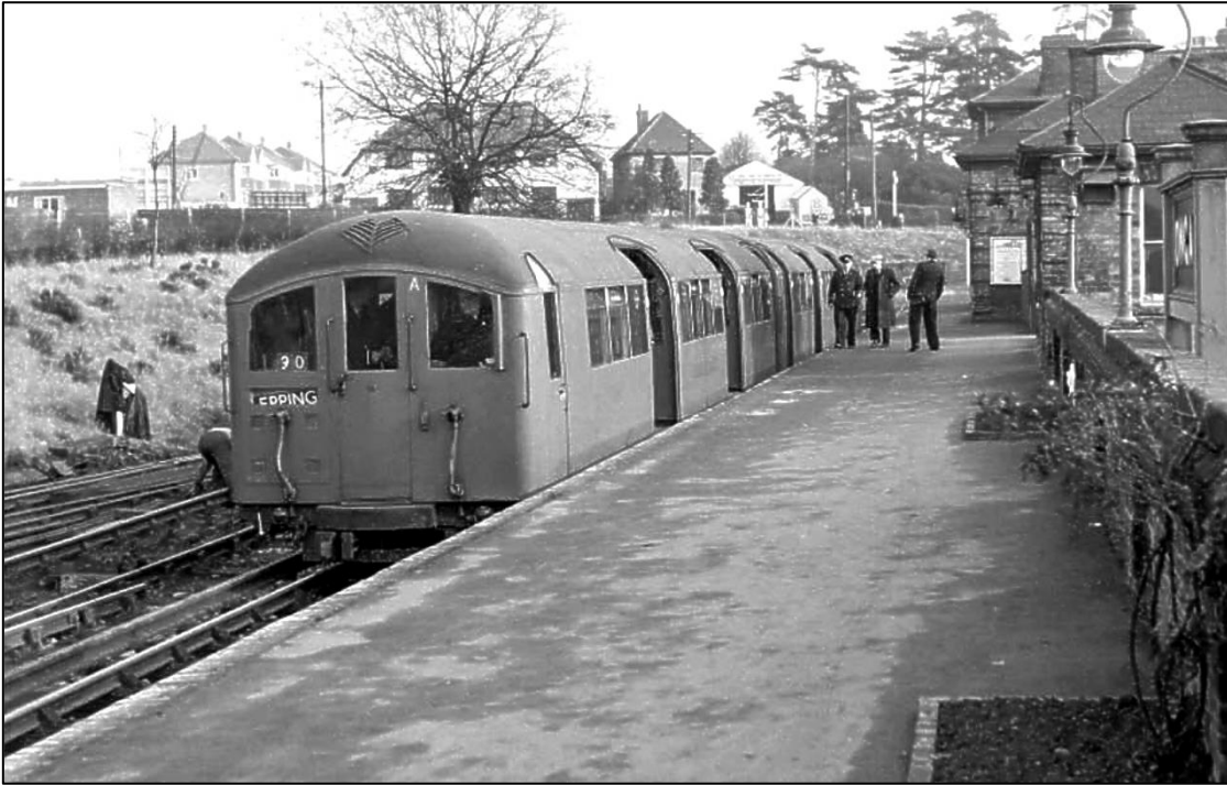
Left: A two-car unit of 1935 Experimental Tube Stock at Ongar in the very early days of electric services. The train has stopped short of the overrun section (see diagram) which was provided to stable a defective unit if necessary. Note at the bottom left, the severed remains of the points, which were used by steam trains to run up to the far end.
